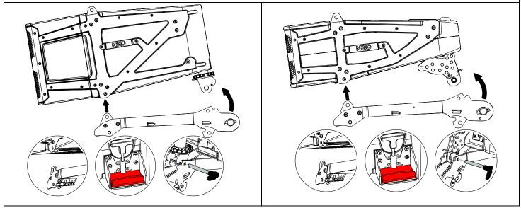
Ensure RedLock<sup>™</sup> safety pins are locked into handle holes. Check rear quick release pins are fully engaged and locked
