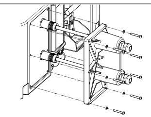
Single Wiring: Place the cable-gland with the O-ring (Ø25) and the cap (M25). Insert the IPCOV, by fixing with the provided screws; Tight the cable-gland to ensure the complete sealing.
