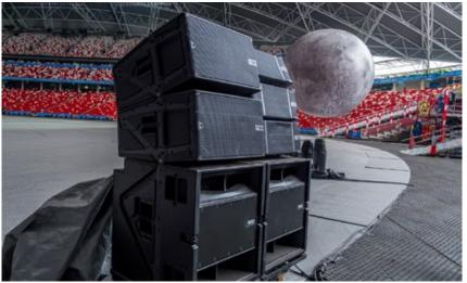
Racks (NUAR) each, with the NUARs flown behind the clusters to keep speaker cables short and lightweight. These covered the top 2 tiers of seating and VIP balconies.
