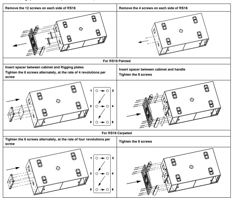
WARNING: Screws must be secured using Loctite 243™
