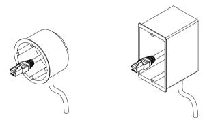
3. Connect the ethernet cable to the NANORM.
