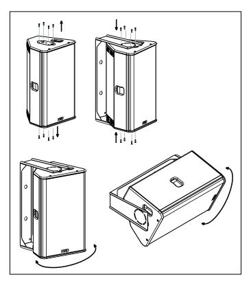
"U" BRACKET MOUNTING PROCEDURE FOR PS15R2
