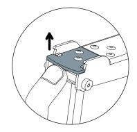
UNLOCKING "U" BRACKET SAFETY LOCKER
