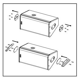
CABLE SUSPENSION MOUNTING PROCEDURE FOR PS15R2
