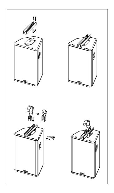
PS SERIES VERTICAL SUSPENSION PROCEDURE
