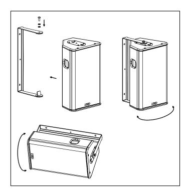
"U" BRACKET MOUNTING PROCEDURE FOR PS10R2
