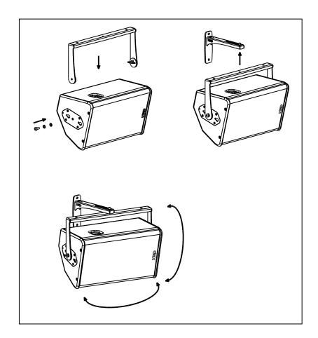
WALL SUSPENSION PROCEDURE FOR HORIZONTAL INSTALLATION
