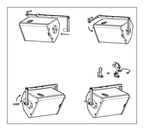
PS SERIES HORIZONTAL SUSPENSION PROCEDURE
