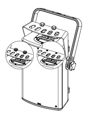
Adjust the P8 and tight properly on the sides, use only fasteners provided.
