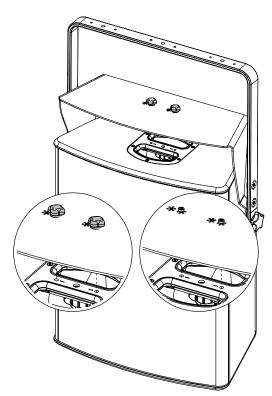
Adjust the P18 and tight properly on the sides, use only fasteners provided.
