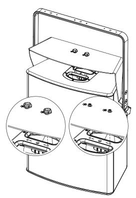
Adjust the P18 and tight properly on the sides, use only fasteners provided.
