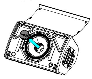
Magnets keep the horn in place.
