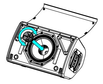
Remove the flange to place the PNU-P8FLG11060.
