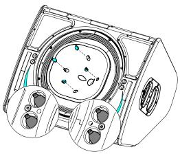
Magnets keep the horn in place.
