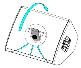
Place the flange, if necessary, rotate it.
