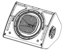
P18-I&TIS Loosen the 3 screws. Remove the grille.
