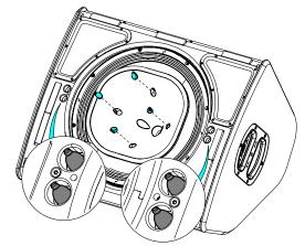
Magnets keep the horn in place.
