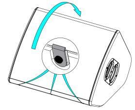
Place the flange, if necessary, rotate it.
