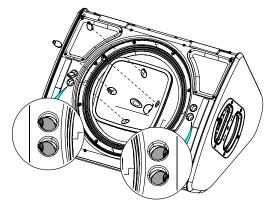
Magnets keep the horn in place.
