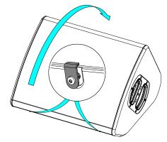
Place the flange, if necessary, rotate it.
