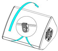
Place the flange, if necessary, rotate it.
