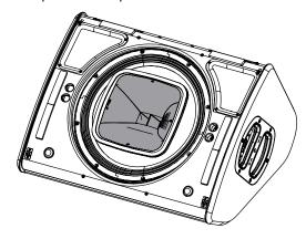
P15-TIS Loosen the 2 screws. Remove the grille.
