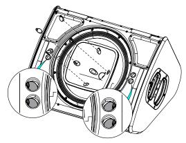
Magnets keep the horn in place.
