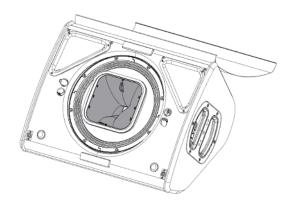
P12-TIS Loosen the 2 screws. Remove the grille.
