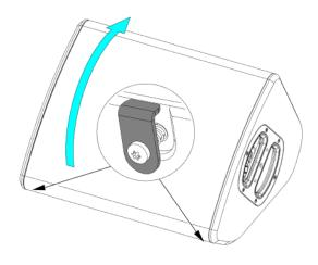
Place the flange, if necessary, rotate it.
