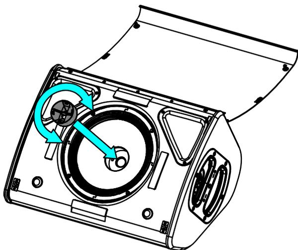
Magnets keep the horn in place.
