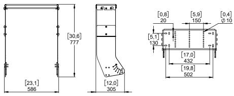
For fixation, you have the choice between M8 and M10 (Fastener not provided)
