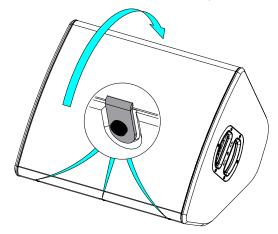
Place the flange, if necessary, rotate it.
