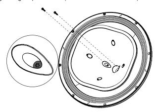
To access to the HF diaphragm, remove 4 screws.
