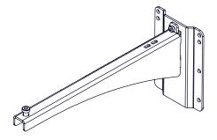
Mount the wall plate. Place the arm in the wall plate.
