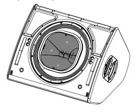
P18-TIS Loosen the 3 screws. Remove the grille.
