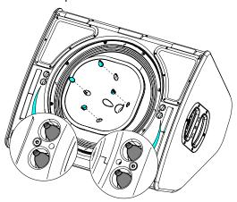
Magnets keep the horn in place.
