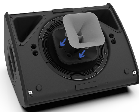
Grille removed, an additional magnetic flange can be quickly fitted to change directivity from 60°x60° to 90°x40°
