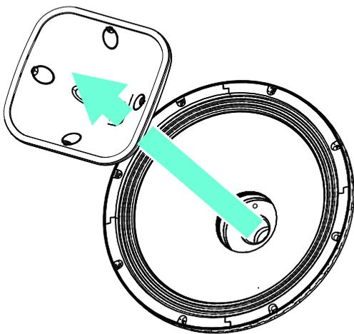
**6** To access to the HF diaphragm, remove 4 screws.
