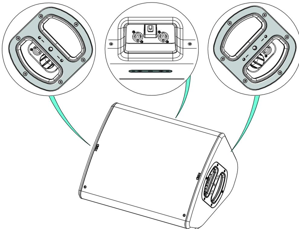
3 locations for connecting, one at the back and one per side.
