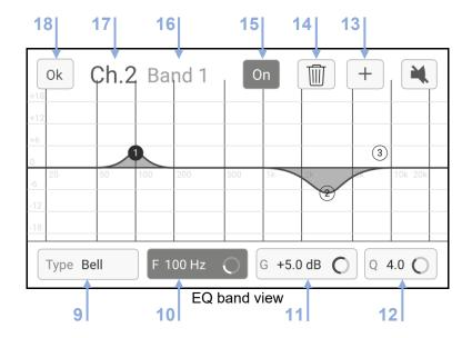
(9) Type of filter, to select between Bell (Parametric), HighPass (2<sup>nd</sup> Order), LowPass (2<sup>nd</sup> Order), HighShelf (with adjustable Q), LowShelf (with adjustable Q) or Notch, from the following popup.
