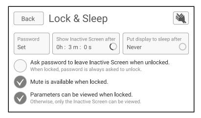
Password is used to lock the screen, the remote-control access (NEXO NeMo or third-party controllers) and the firmware update (NEXO NeFu). Using a password in not mandatory and can be left empty.
