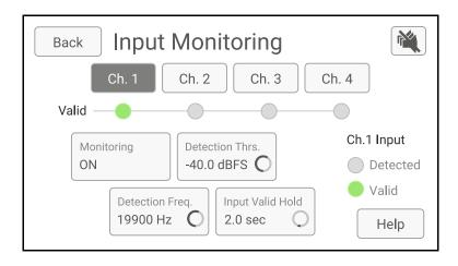
This menu allows setting up all the NXAMPmk2 Input Monitoring parameters per channel. Basically, this monitoring function measures the pilot tone presence on the amplifier channel input at one frequency point and can report an alert ("Valid" input pilot tone detection) if the pilot tone is not detected.
