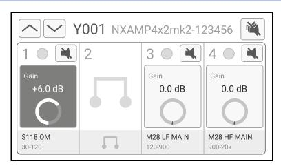
Select a channel (button is highlighted), then turn the wheel to change the gain setting.
