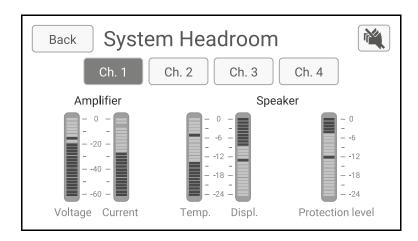
The System Headroom menu displays for each channel (selected by the top buttons Ch.1 to Ch.4) the headroom available from both the amplifier channel and the speakers connected to it.
