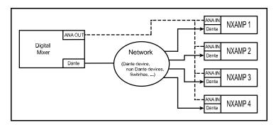
If for example, the NXAMPmk2 n°2 does not received the audio packets from the subscribed source (here the mixer) then it will unmute the analog inputs, as shown below.
