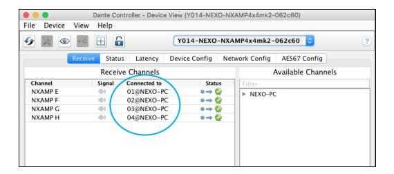
The digital audio status for the NXAMPmk2 is declared OK if all digital input channels E/F/G/H are declared OK, otherwise all analog inputs are un-muted.
