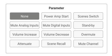
Then choose a parameter (see table below, e.g. Switch Scene), then if needed a first and a second option (e.g. the Scenes to switch). Finally, choose if this action should be triggered when the pin's state is high, low, or on impulse (there is no threshold).
