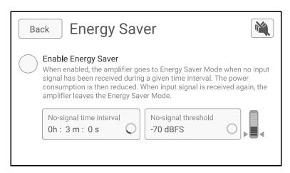
No-signal time interval can be adjusted from 1 minute to 3 hours.
