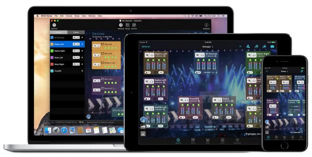
Managing and positioning amplifiers, monitoring their parameters (levels, etc.), and setting new values (preset, volume, delay, EQ, etc.) is made possible thanks to an attractive and intuitive user interface. NEXO NeMo also comes with a powerful engine for logging, alerting and emailing.
