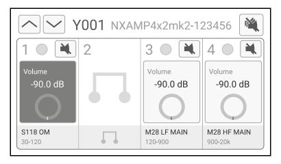
Select a channel (button is highlighted), then turn the wheel to change the volume setting. You can select multiple channels, when a selected channel reaches the maximum value, it will cease to increase by continuing to turn the wheel, but other selected channels may still increase the setting; Be careful not to change a gap between two channel settings when selecting multiple channels at the same time.
