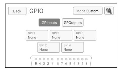
The five LEDs to the left at the bottom of the screen are real-time monitoring the values of the input pins of the NXAMPmk2's GPIO port (Gray means low, Green means high, i.e. +5V).
