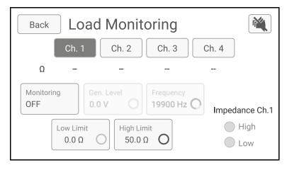
This menu allows setting up all the NXAMPmk2 Load Monitoring parameters per channel. Basically, this monitoring function measures the impedance on the amplifier channel at one frequency point and can report
