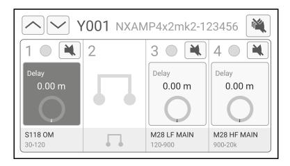
Select a channel (button is highlighted), then turn the wheel to change the delay setting.
