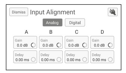
Select the gain or delay you want to modify and turn the rotary encoder to adjust the value. Gain range is from -6dB to 6dB and delay range is from 0.00ms to 10.00ms. When input alignment is active (different from 0dB and 0.00ms), a small reminder icon is displayed on the concerned input on the input patch page.
