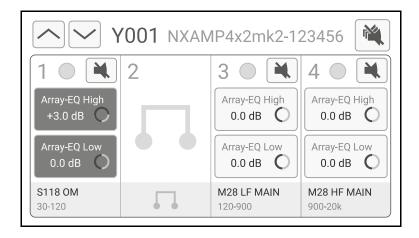
Select an Array-EQ in a channel (button is highlighted), then turn the wheel to change the Array-EQ setting.
