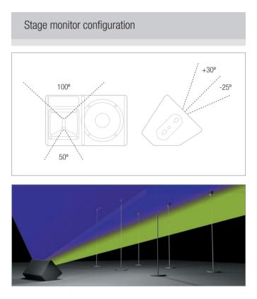
In stage monitor mode, a PS R2 Series loudspeaker yields 100° horizontal coverage at 30° above the centre line, narrowing to 50° horizontal coverage at 25° below the centre line for use when the performers are further away.
