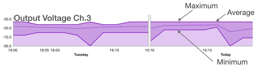
Each graph contains three curves, one for the maxima, one for the minima, and one thinner for the average. The small gray spaces between curves are for the moments where the log was not being recorded (on the picture above, for instance, log was not recorded between Tuesday at 18:15 to Today at 10:10).
