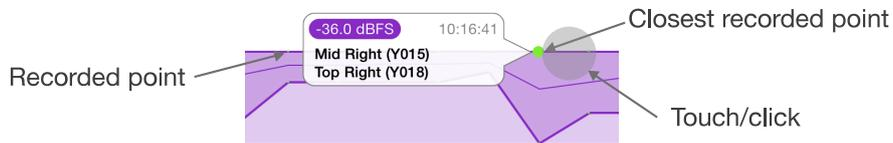
Put your finger/click near a curve. The recorded points are displayed in another color, and a bubble appears to give detail about the closest point to which your finger/the mouse is. It contains the value, the date, and the NEXO device(s) realizing this value at that date. Slide to see the details about other points.
