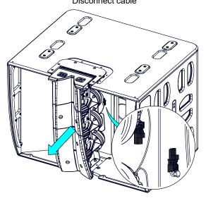
Remove 4 screws to access diaphragm.
