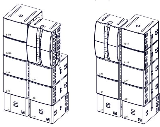
Tilt the unit so that the vertical HF dispersion axis is parallel to the audience floor.
