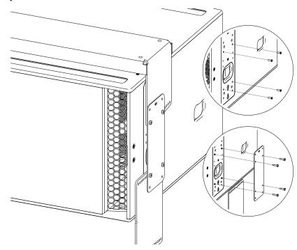
Warning: Use only provided screws (thread lock coated or use Loctite 243).
