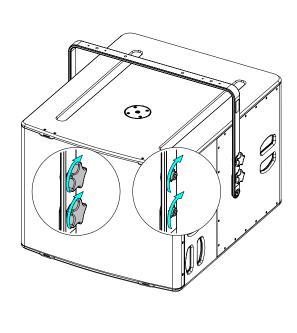
Place on CLADAPT, use the 2 guides. Tight with the fasteners provided with CLADAPT
