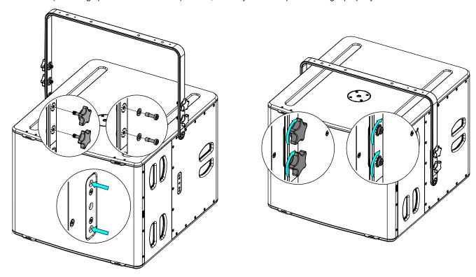
Place on CLADAPT, use the 2 guides. Tight with the fasteners provided with CLADAPT
