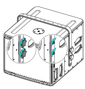
Place on CLADAPT, use the 2 guides. Tight with the fasteners provided with CLADAPT
