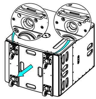
Push the 2 latches and lock the Wheelboard.
