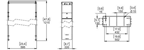
For fixation, you have the choice between M8 and M10 (Fasteners not included)
