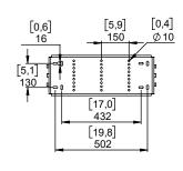
For fixation, you have the choice between M8 and M10 (Fasteners not included)
