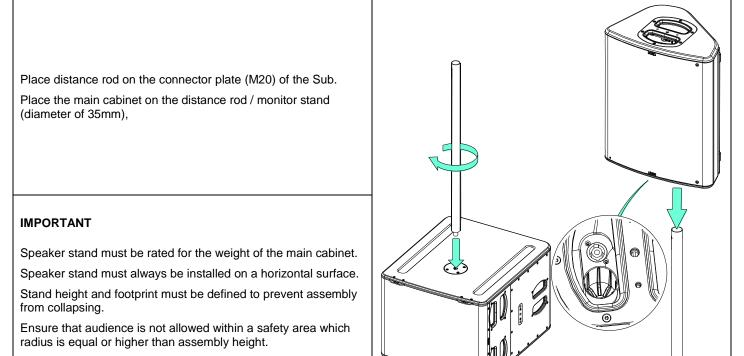
Test steadiness of the assembly by pushing in all directions.
