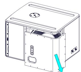
Remove the driver. Tightening torque: 3.5 Nm (Thread Locker: Loctite 242)
