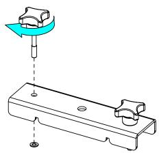
Mounting of a hook on the accessory (fasteners not provided). For 10mm (0.4 inch) diameter fasteners.
