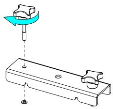
Mounting of a hook on the accessory (fasteners not provided). For 10mm (0.4 inch) diameter fasteners.
