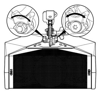
Tilt: Loosen the wing nut to adjust the angle (-45° to +45°).
