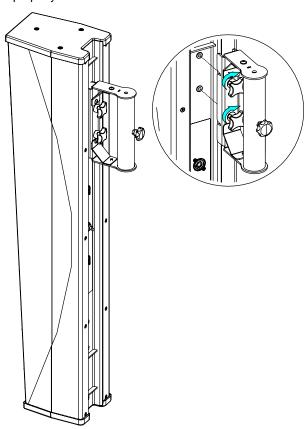
Place the assembly on the pole stand, tighten the knob to maintain the desired orientation.
