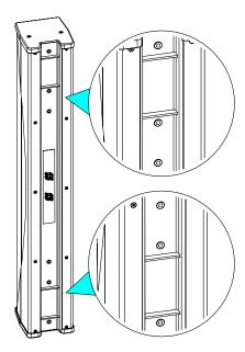
2 locations for connecting, 1 on the back and a quick connect in the base cover (ID84 only).
