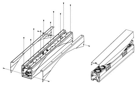
Remove the 4 screws and the RJ45 connector. Remove the HF assembly. Tx20
