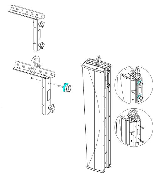
For Touring use, place the knob through the part and screw the washer on it. Tight properly.
