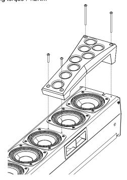
Remove the 4 screws to access the 4-inch driver. Tx15 Tightening torque: 1.0Nm
