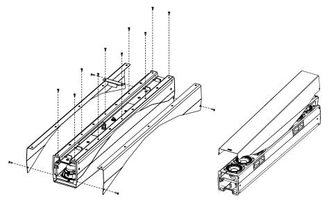
Remove the 4 screws and the RJ45 connector. Remove the HF assembly. *Tx20 Tightening torque : 1.2Nm*
