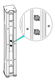
ID84 versions T & TIS: a directivity switch, located between the NL4 connectors, allows to virtually curve the drivers to achieve 2 vertical directivity patterns:
