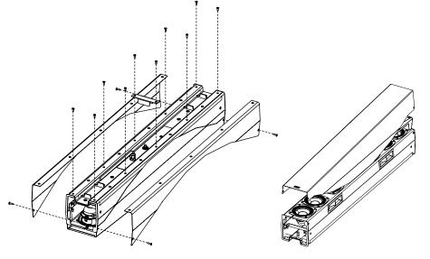
Remove the 4 screws and the RJ45 connector. Remove the HF assembly. *Tx20 Tightening torque : 1.2Nm*
