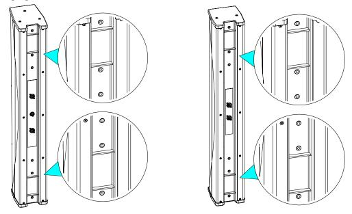
2 locations for connecting, 1 on the back and a quick connect in the base cover (ID84 only).
