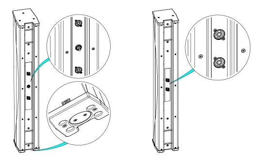
ID84 versions T & TIS: a directivity switch, located between the NL4 connectors, allows to virtually curve the drivers to achieve 2 vertical directivity patterns:
