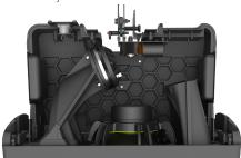
Internal view of the GEO M10 module, showing from left to right the HWR<sup>™</sup> waveguide, the Neodymium 10" with PDD<sup>™</sup> devide and the curved V-shaped port.
