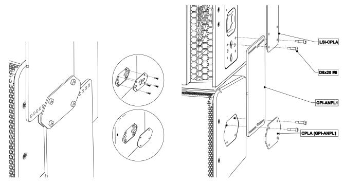
Warning: Use only provided screws (thread lock coated or use Loctite 243).
