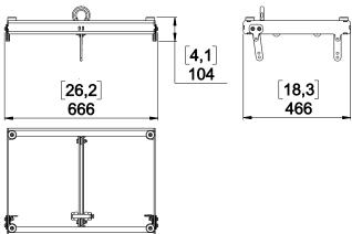
Use: Max 12x GEOM12 flown on one or two rigging points or 3x GEOM12 stack.
