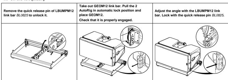
WARNING: Use shackle model: Alloy Bolt Type Shackles 3.25 Tons Use NEXO Simulation Software for mechanical prediction
