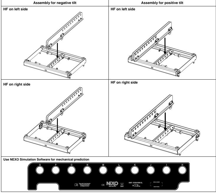
WARNING: Use shackle mode: Alloy Bolt Type Shackle 3.25 Tons Use NEXO Simulation Software for mechanical prediction
