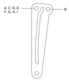
SAFETY: You can replace one of the four screws with an eyebolt (M8) and use a sling (apply thread lock on the eyebolt).
