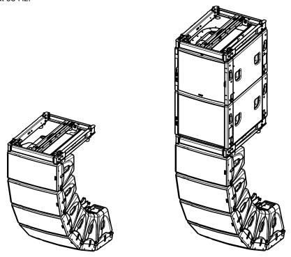
For long throw stacking application on floor or on MSUB15, up to 6 boxes used at 63 Hz without Sub and 85 Hz with MSUB15 at 85 Hz.
