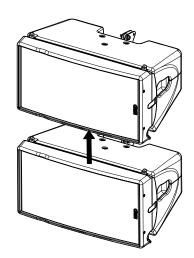
Connect both cabinets by inserting the axis through front holes and secure axis with brake nuts.
