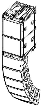
For long throw stacking application on floor or on MSUB15, up to 6 boxes used at 63 Hz without Sub and 85 Hz with MSUB15 at 85 Hz.
