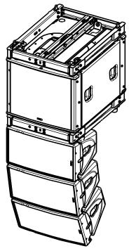
Possibilities to use 2-3Box setup in stack configuration using MSUB15 in OMNI or CARDIO mode with 1 Back and 2 front and 3 GEOM10 on top of them, application venue up to 15 meters, default cross over 85 Hz but small overlap could have impact if needed, for example (MSUB15 120 Hz and GEOM10 75 Hz).
