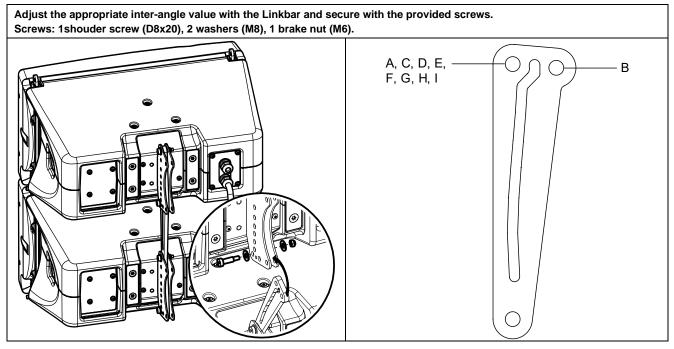
SAFETY: You can replace one of the four screws with an eyebolt (M8), and use a sling (apply thread lock on the eyebolt).
