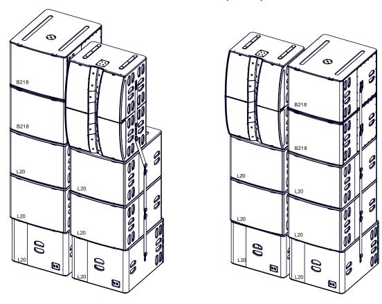
Tilt the unit so that the vertical HF dispersion axis is parallel to the audience floor.
