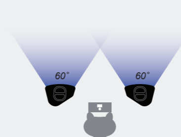
Simple System: 2 x P12 with standard horn
