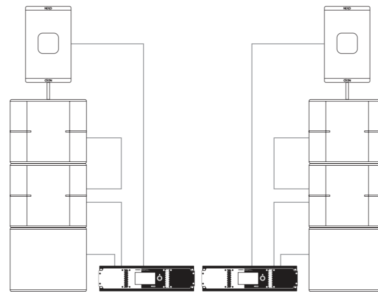
Mid-Sized FOH System: (Per side) 1 x P15 (Active) on 2 x L18 Subs on 1 x L18 Sub (Cardioid Mode), powered by 2 x NXAMP4X4MK2
